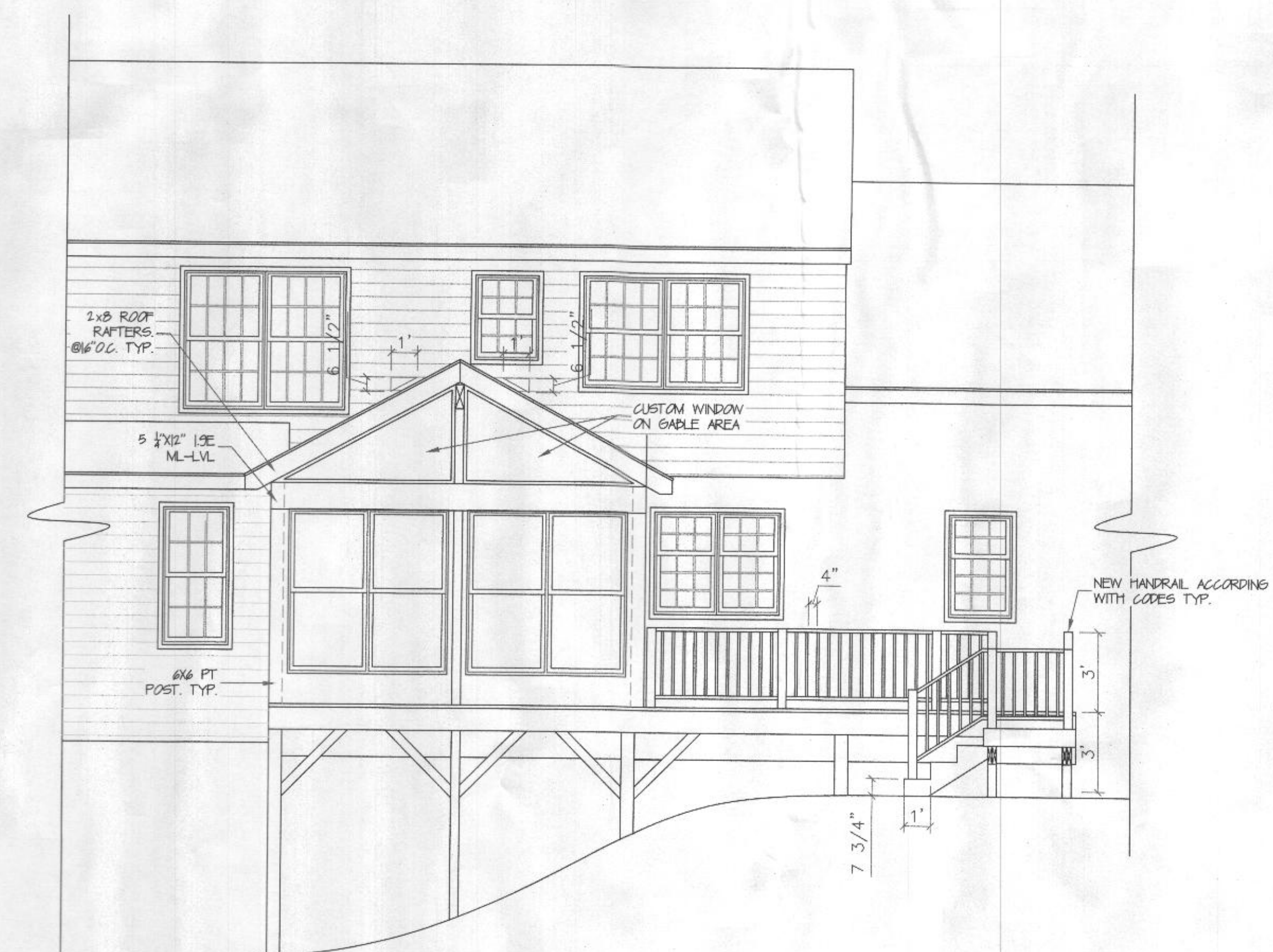
EXISTING & PROPOSED REAR ELEVATION 1/4"=1'-0"
