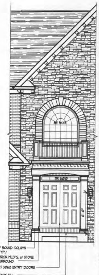
FRONT ELEVATION #3A SCALE: 1/8" - 1/4" = 1'-0" SHOWN W/ OPT. DUAL DOOR ENTRY
