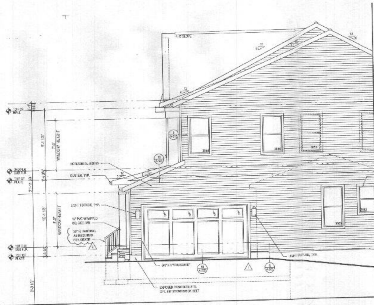
4 PART. RIGHT SIDE ELEVATION w/ OPT. 012 - SIDE LOAD GARAGE SCALE: 1/4"=1'-0" ELEV. 2 - SHOWN
