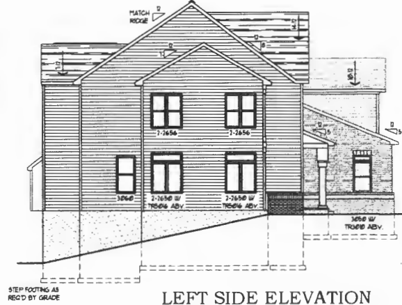
LEFT SIDE ELEVATION SCALE (17x11) 1/16" = 1'-0" SCALE (18x24) 1/8" = 1'-0"
