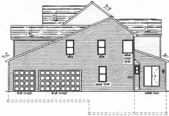
RIGHT SIDE ELEVATION SCALE (17x11) 1/16" = 1'-0" SCALE (18x24) 1/8" = 1'-0"
