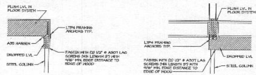
ATTACHMENT DETAIL SCALE: 1/2" = 1'-0"
